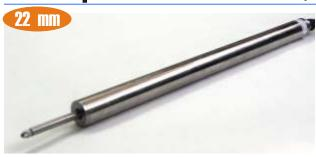
The DS Series of DC LVDTs are range of DC-input DC-output displacement transducer housed in stainless steel body. These transducers are equipped with in-built electronics. Output of ±5V or 0 to 10 V makes them very easy to use and apply. No external signal conditioner or amplifier is required for there operation.
