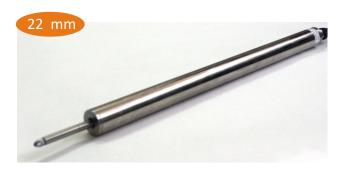
These AC LVDTs are the most economically priced displacement transducers. Housed in stainless steel body, they are a combination of ruggedness and high performance.
