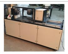
TSTM is a line of microprocessor controlled motorized machines designed to automate, simplify and standardize the strength different types Torsion Springs and different specimen both in clockwise and counterclockwise direction. Electronics Torque Transducers are used measure the torque and optical encoders to measure angle of rotation accurately.
