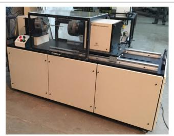
Models TSTM-200 TSTM-500 and TSTM -1000 and TSTM-2000 are High Torque models. They incorporate imported Precision **Torque Transducer.**
